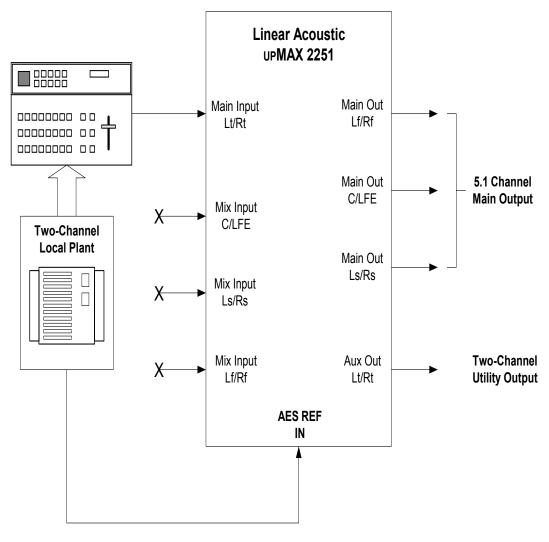
Figure 3-1 UPMAX 2251 in a commercial upmixing application
