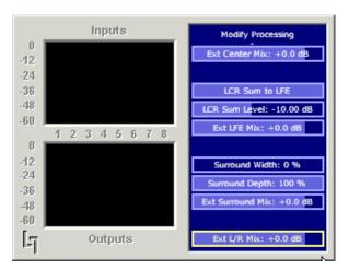
Figure 4-2 Modify Processing menu; scroll down to access Ext L/R Mix (as shown on right menu)
